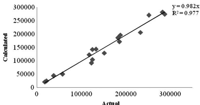
FIG. 4. Correlation between actual and calculated data for validation of special cubic model of formulations viscosity.
