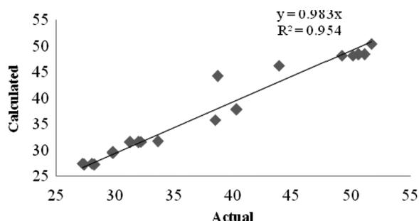
FIG. 2. Correlation between actual and calculated data for validation of linear model for surface tension.
