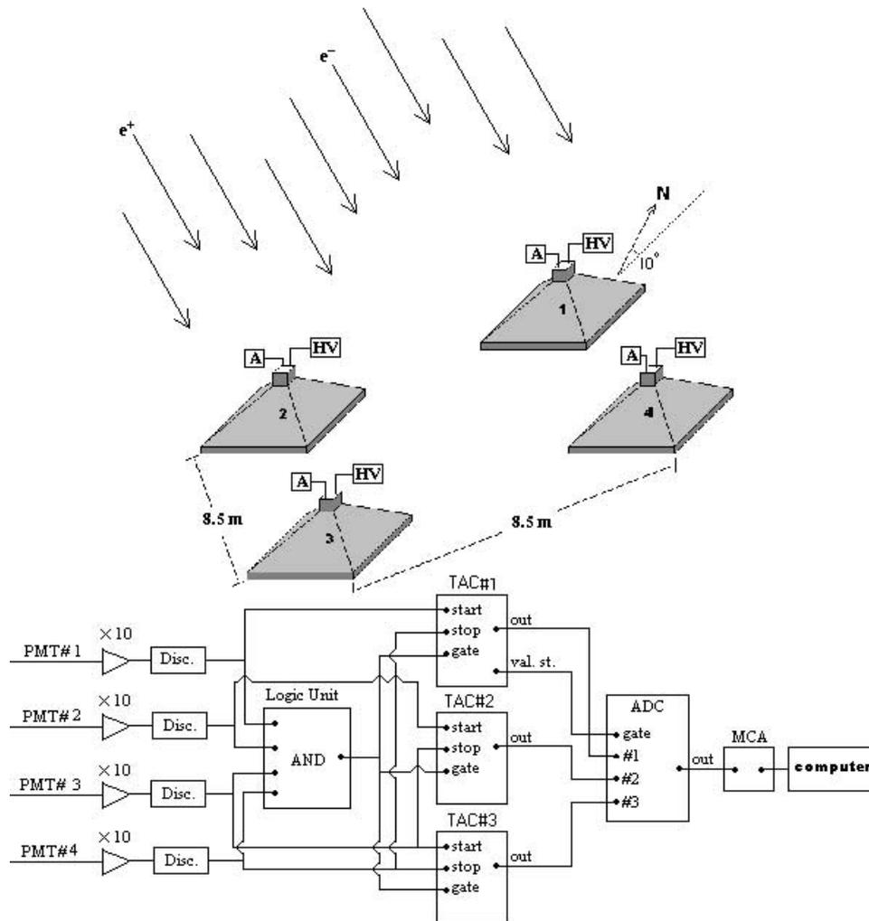
Figure 1. Arrangement of four scintillators as a square array, and its electronic circuit.
