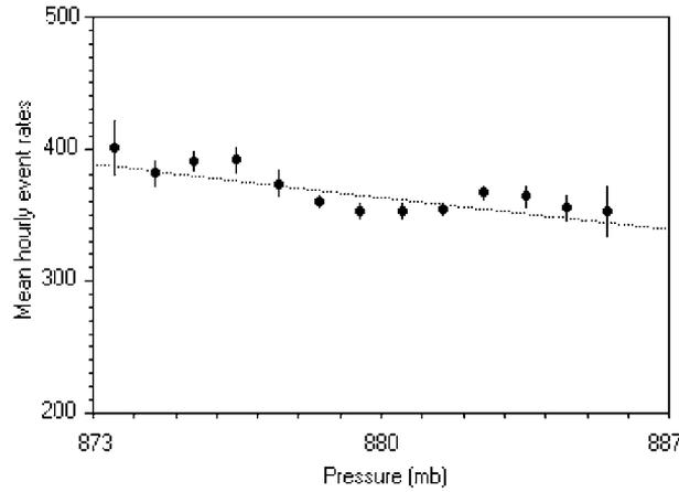
Figure 3. Mean event rates, over all zenith and azimuthal angles and all times, as a function of atmospheric pressure.
