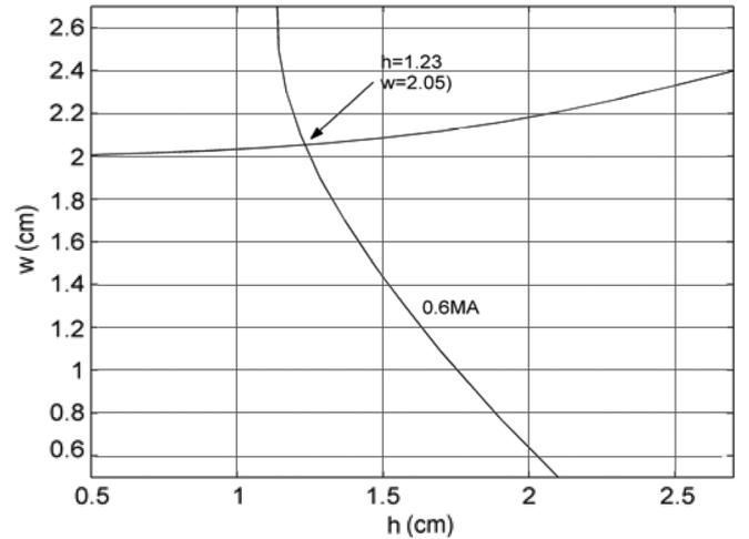
Fig. 4. Determination of the optimum dimension of rail in 0.6 MA.
