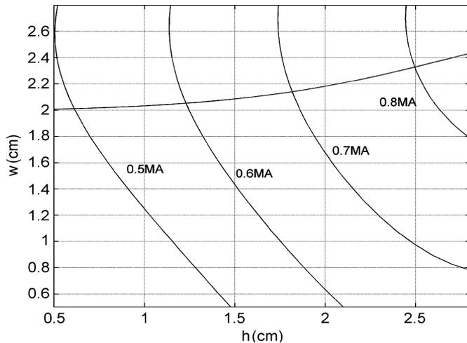
Fig. 5. Optimum dimension of rail for 0.5, 0.6, 0.7, and 0.8 MA.
