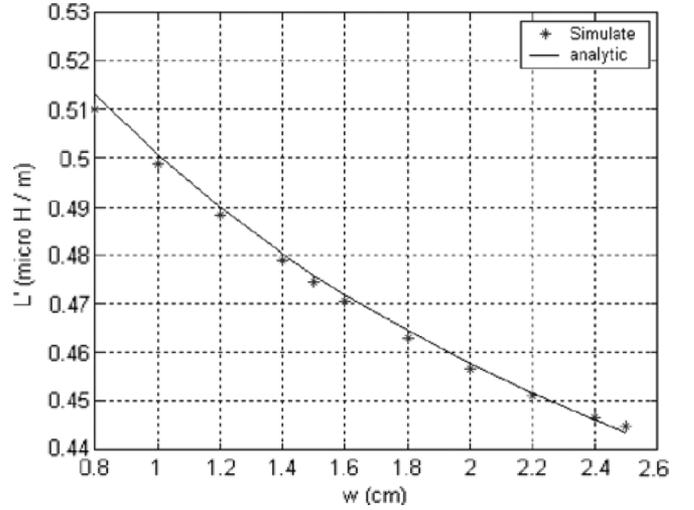
Fig. 3. Comparison of analytical phrases and simulation for  $h = 2$  cm. Simulation: \*. Analytic: —.
